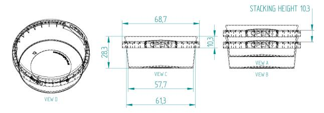
TAMPER EVIDENCE Tamper evidence break-out tab
