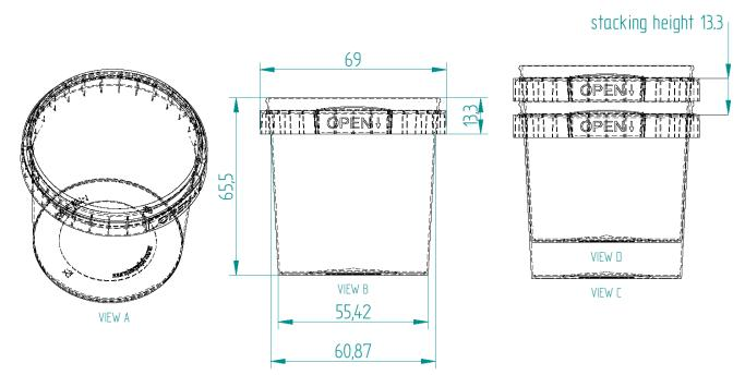
TAMPER EVIDENCE Tamper evidence break-out tab
